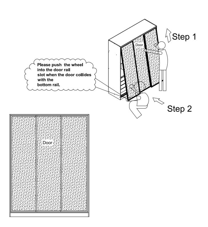
Normally the vertical edge of door should be aligned with the wardrobe side panel. Refer to below instruction if it's not.
