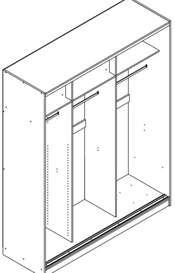
Please note – Some floors could possibly not be level or flat so it is best to ensure the wardrobe carcass frame is square and level prior to fitting of doors. This might involve the use of packing material under the base.
